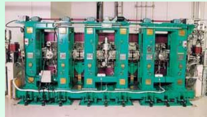
In-vacuum type NdFeB magnet undulator
